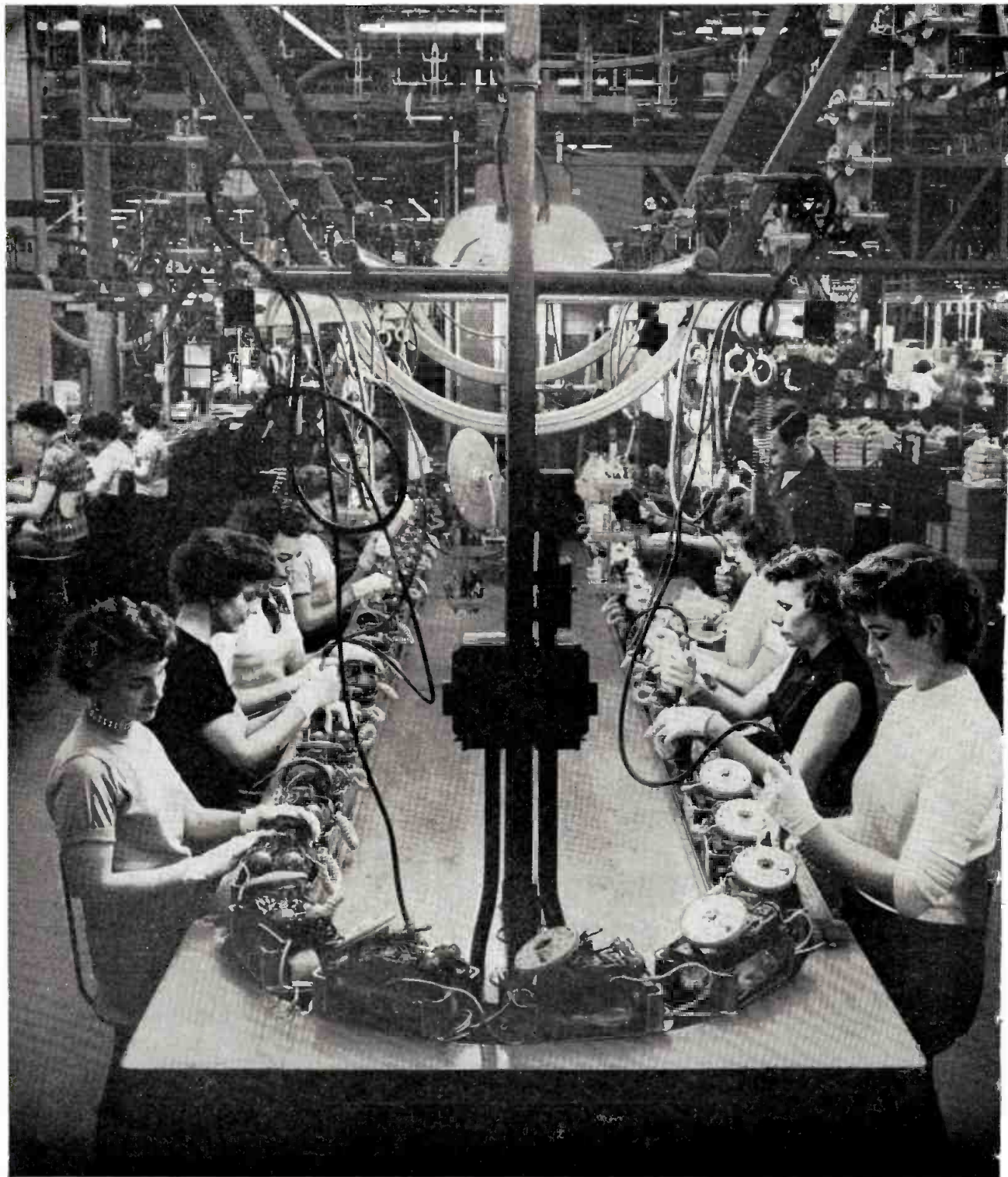
TELEPHONE TEAMWORK. At Western Electric's Indianapolis Works, these girls handle the final assembly of telephone sets. A 2½-mil long conveyor system links the various manufacturing steps, bringing components and sub-assemblies from every corner of the plant.
